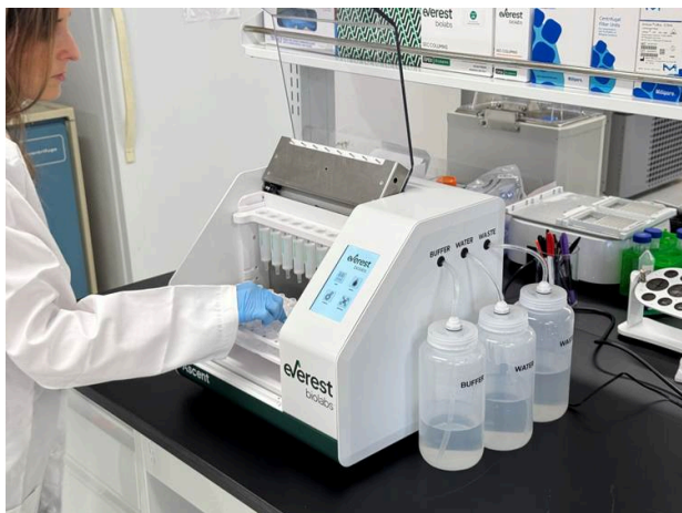
Figure 2. The Ascent instrument. Parallel, hands-free SEC-based EV isolation for up to 8 samples at a time.
